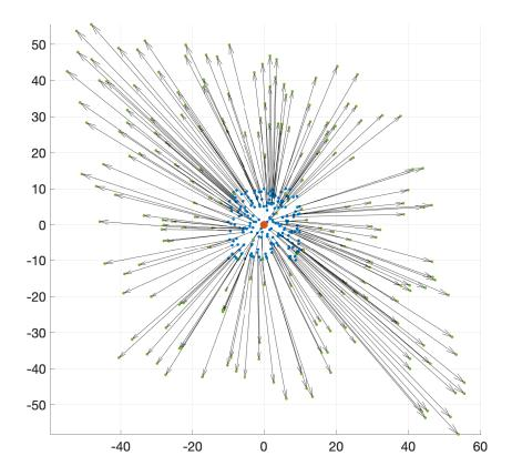
It already gives us a sense: The arrows are all pointing outwards, showing that **A** perform some sort of enlargement (scaling with a scale k > 1). But this enlargement is not uniform, it is more pronounced along a NorthWest-SouthEast axis. Notice that this NorthWest-SouthEast axis can be described by the vector
